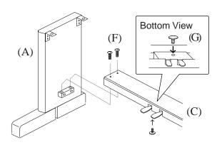
1. Insert the Adjuster (G) on the bottom of Pedal Board (C). Fasten (A) and (C) with four bolts (F).
